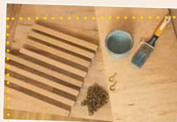
First saw the boards into uniformly sized pieces: Four of the pieces should be as long as the short side of the board. The other four pieces can be a little bit longer.
