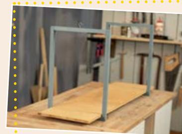
Set up the frames and push the board through so that it receives stable support from both brackets. Screw one hook into each top of the frame, attach the chains, and hang the shelf on the ceiling – wow!
