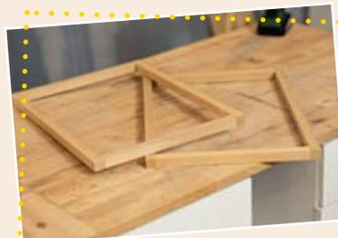
Drill holes into the ends of the boards and connect them to form two identical frames using the screws. Paint the frames if desired.
